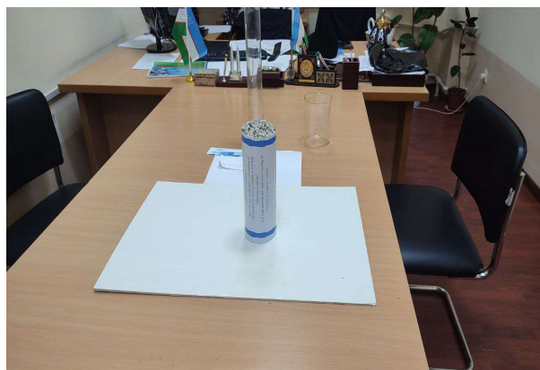
Figure 7. Determination of the fuzzy seed repose angle
