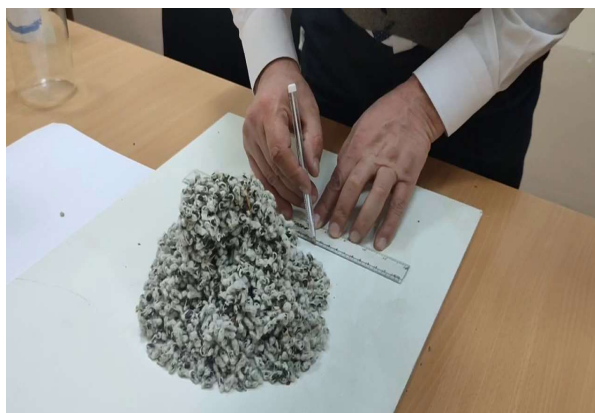
Figure 7. Determination of the fuzzy seed repose angle
