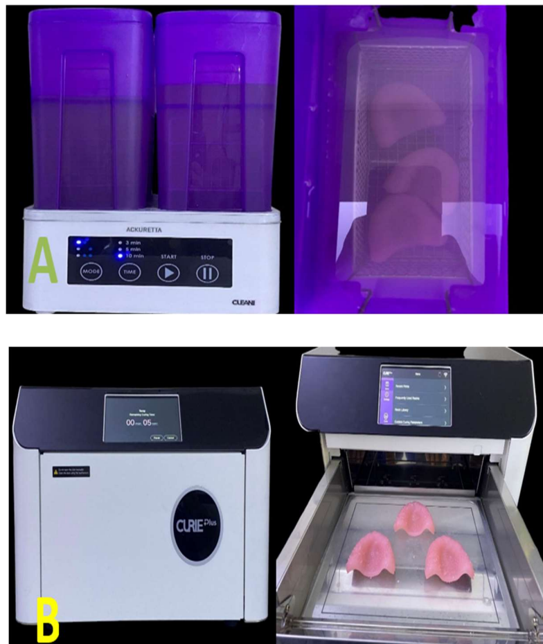
Figure (6): A, 3-D printer denture base in isopropyl alcohol. B, 3-D printer denture base treated with ultraviolet light post polymerization machine
