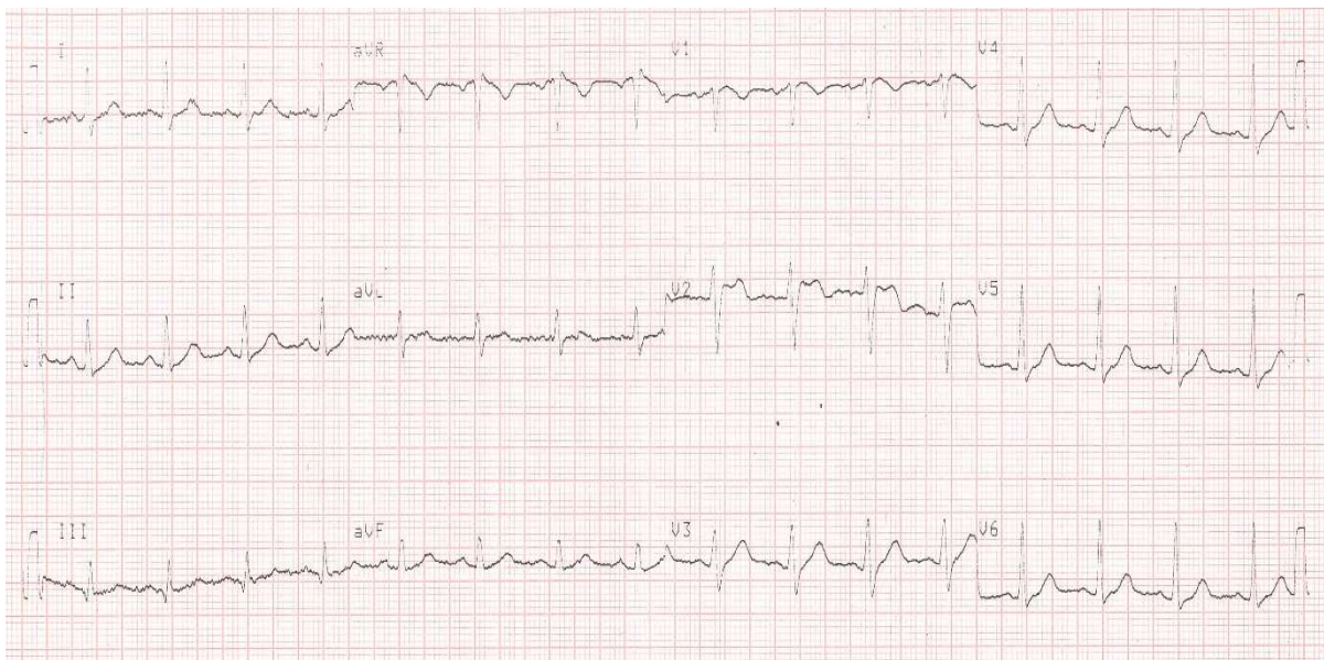
Fig 3. The healthy & resting ECG signal response of commercial Ag/AgCl ECG electrode, Pristine Graphite base and Graphite MWCNT hybrid Electrodes
