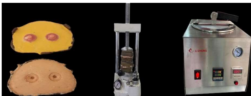
Figure 7: Curing the specimens of shear bond test after relining
