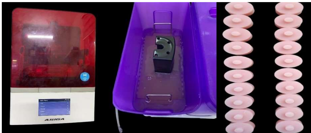
Figure 3: Asiga printer used for 3D printing specimens of shear bond
