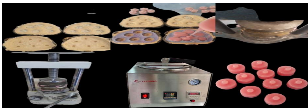
Figure 5: Curing the conventional heat cured specimens of shear bond test
