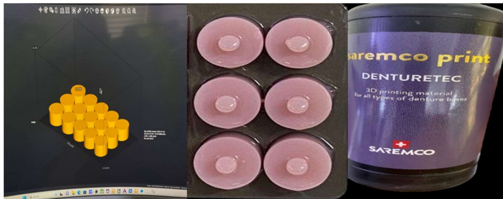
Figure 2: Saremco Materials used for 3D printing the specimens of shear bond
